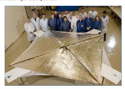
**Above:** The Huntsville-based NanoSail-D team stands with the fully deployed sail at ManTech SRS technologies on April 16, 2008, after the successful deployment test.
