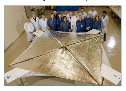
Above: NanoSail-D poses after a successful laboratory deployment test: movie.
