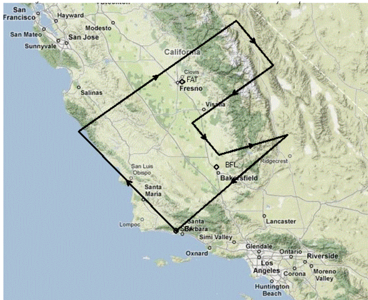
Figure 5.1.4: Sample Twin Otter flight plan. Flight duration is 5 hours and distance covered is approx. 700 nautical miles.
